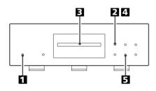
1 Turn on the power using the POWER button on the main unit.
